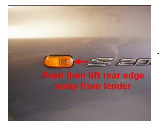
5. Remove the side turn signal housing by pushing it towards the front of the car and lifting the rear edge away from the fender. The lamp housing is held in place by a plastic spring clip that is molded into the front edge of the housing. Be careful – with age the plastic spring clip at the front edge can get brittle and if you push too hard it may crack or break. Push only far enough to get the rear of the housing free of the fender, and then the entire housing will come out.
