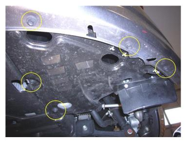
Starting at the front edge, pull the fender liner down so you can reach the headlight and side turn signal wires.
